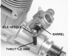
The engine will accelerate from idle to full throttle smoothly and instantaneously when properly adjusted. The engine may not idle well at a low setting or accelerate as quickly until it is well broken in.
