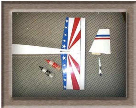
Put epoxy on the bottom of the vertical stabilizer and slip it into its slot. While the epoxy is setting, use a triangle or a builder's square to make sure that the vertical stabilizer is aligned 90 degrees to the horizontal stabilizer. After the epoxy sets, use CA to glue the sides of the vertical stabilizer to the top of the fuselage.
