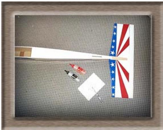
Glue the horizontal stabilizer into its slot with five-minute epoxy. Recheck the alignments frequently until the epoxy sets. After the epoxy has cured, remove the wing from the fuselage.
