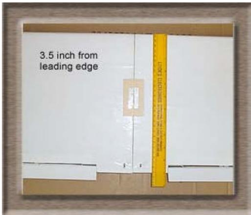
front of the wing, and draw a line around the tray on the surface of the wing. Remove the covering material from within the lines and glue the tray in place. Working through the opening in the tray, use a rotary grinder or hobby knife to cut a hole in the wing surface and the center ribs to clear the servo. Now feed the servo wire between the tray and the wing surface and install the servo with the servo wheel toward the rear, using the directions, which came with the radio.
