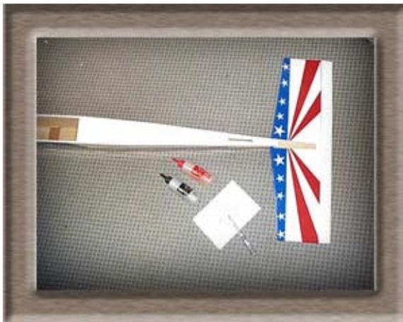
Glue the horizontal stabilizer into its slot with five-minute epoxy. Recheck the alignments frequently until the epoxy sets. After the epoxy has cured, remove the wing from the fuselage.
