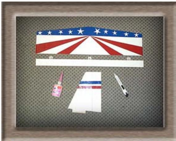
Mark the center of each hinge and insert them in the front of the ailerons, using the mark to make sure that the hinges only go in one half of their length. DO NOT GLUE THEM YET. Push a straight pin through each hinge on the center mark. Now fit the ailerons by inserting the hinges into the back of the wings and the aileron torque rods into the predrilled holes in the ailerons.
